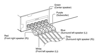
**2** Connect the speaker cord with the color tube to  $\oplus$ , and the speaker cord without the color tube to  $\ominus$ .
